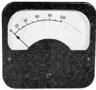
Volume Unit Meter. Used in programme input equipment in the U.S.A. and elsewhere
