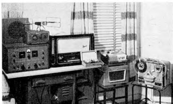
Kenneth Miller's equipment includes shortwave receiver, Panadaptor (for visually examining incoming signals), directional FM antenna, AM/FM receiver, three standard recorders and a battery portable
