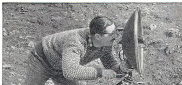
Parabolic reflector fitted with gun-sight gets it all on Emitape. E. D. H. Johnson, the expedition's recordist, used this special equipment to record the songs of distant birds.
